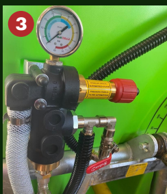
3 Constant pressure regulator. With integrated Autofilter.
