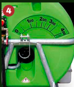
4 Chemical tank. Tank contents by large index.
