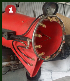
1 Flexigun Cannon Sprayer and Electrostatic. Easy to adjust for vertical or horizontal spraying.
